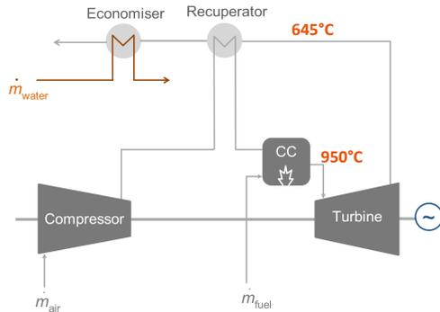
Higher quality recuperator materials are necessary to fully exploit the potential for humidification
