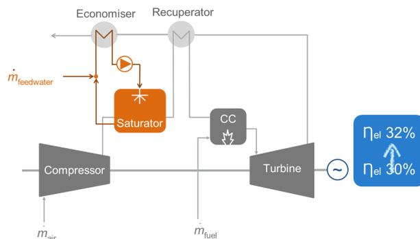
The mHAT concept was experimentally tested and validated in our test rig.
