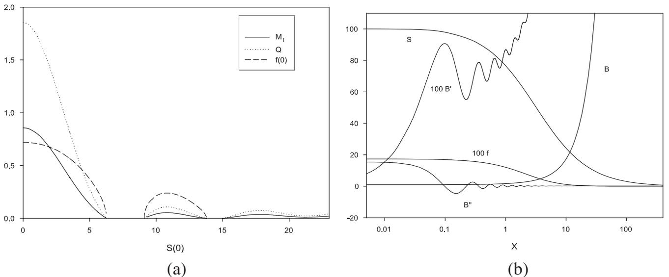
FIG. 12. Boson stars in the scalar-tensor theory corresponding to  $\lambda = 1$ ,  $\nu = \mu = 0$ ,  $\kappa = 0.1$ . (a) mass, particle number  $Q$  and the value  $f(0)$  as a function of  $S(0)$ ; (b) details of the profile for  $S(0) = 100$ . The high value of  $S(0)$  was chosen to get noticeable oscillations—see the text.
