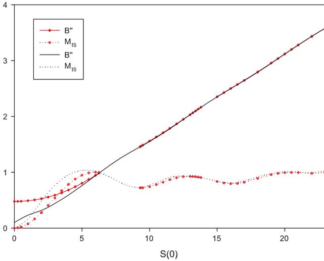
FIG. 13 (color online). The value  $B''(0)$  and the inertial mass of the field  $S$  for STBS (online red) and STR soliton (online black) as functions of  $S(0)$ . Notice the gaps in the STBS (red) curves where no solutions exist. This can be used to distinguish between the cases in a black and white plot.
