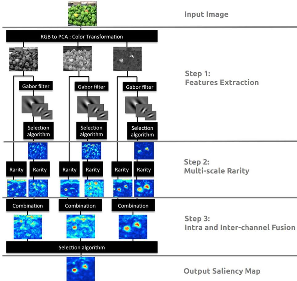
**Fig. 1.** Diagram of our proposed model. First, from the input image, colour and orientation features are extracted in parallel or sequentially. Then, for each feature, a multi-scale rarity mechanism is applied. Finally, two fusions (intra- and inter-channel) are made from the rarity maps to provide the final saliency map.
