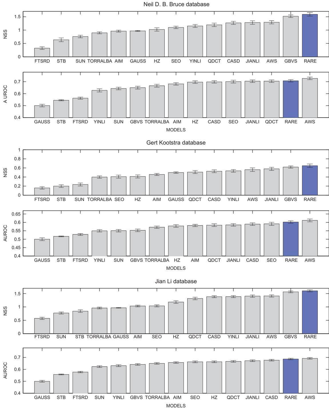
**Fig. 9.** Comparison of our model with 13 state-of-the-art saliency models and a centred Gaussian. The first two graphs display the NSS and AUROC metrics for the Toronto dataset. Graphs 3–4: for Kootstra dataset. Graphs 5–6: for the Jian Li dataset. RARE2012 outperforms the other models for the NSS metric and is the second best for AUROC metric.
