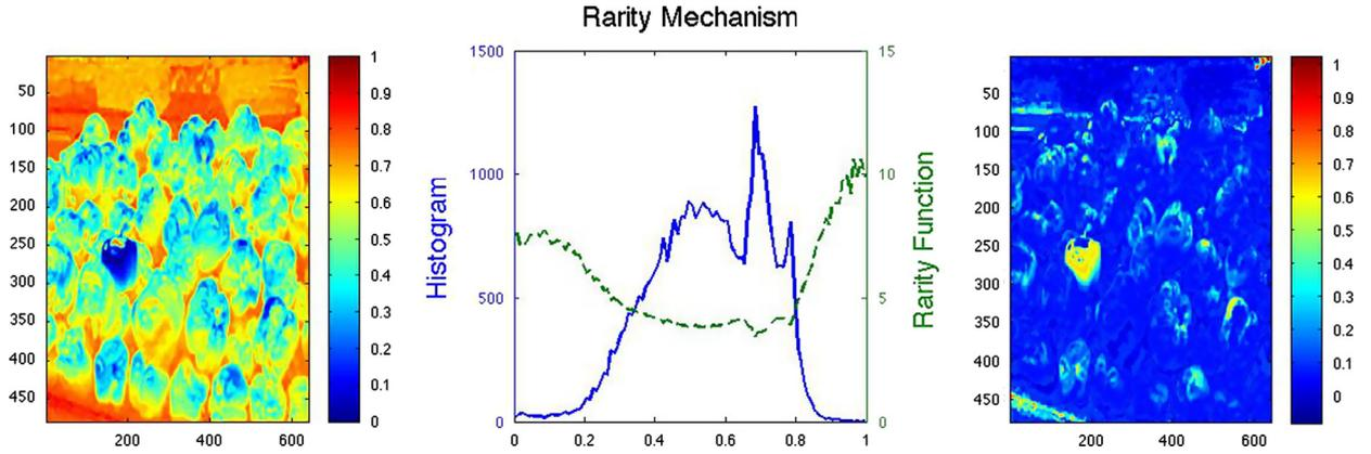
**Fig. 2.** Illustration of the rarity mechanism on a single scale. Rarity function (green curve in the middle graph) is computed from a histogram (blue curve) of a feature map (left image) to a given scale. This process is repeated at several scales. Output is a reconstruction of the map where high values are given for the most “rare” areas (right image).
