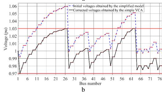
**Fig. 4.** The voltages obtained using simplified network component models as well as boxplots of initial and corrected voltages considering the uncertainty associated with the voltage dependency of loads (a) in the voltage drop case, (b) in the voltage rise case
