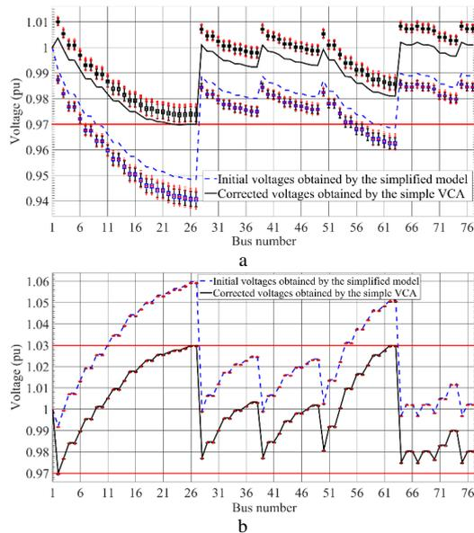
**Fig. 5.** The voltages obtained using simplified network component models as well as boxplots of initial and corrected voltages considering the uncertainty associated with the power factor of loads (a) in the voltage drop case, (b) in the voltage rise case
