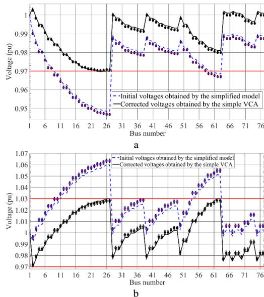
**Fig. 8.** The voltages obtained using simplified network component models as well as boxplots of initial and corrected voltages considering the uncertainty associated with the internal resistance of transformer (a) in the voltage drop case, (b) in the voltage rise case
