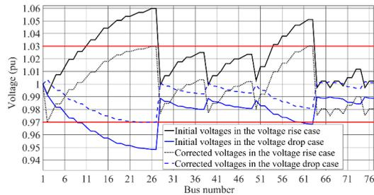
**Fig. 3.** Initial nodal voltages as well as the corrected ones obtained by the simple VCA relying on the simplified deterministic models of network components
