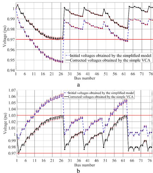
**Fig. 6.** The voltages obtained using simplified network component models as well as boxplots of initial and corrected voltages considering the uncertainty associated with thermal dependency of lines (a) in the voltage drop case, (b) in the voltage rise case
