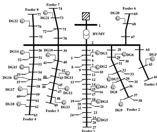
Fig. 2. 77-bus radial distribution system
