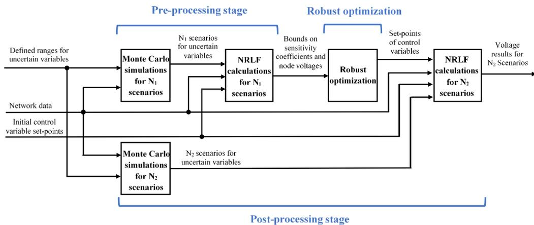
Fig. 1. The proposed approach to develop the robust voltage control algorithm
