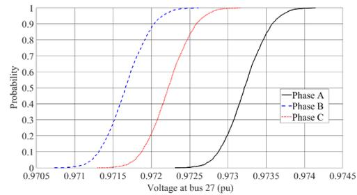
Fig. 10. The CDFs of three phase voltages at bus 27 obtained by the RVCA in the voltage drop condition.
