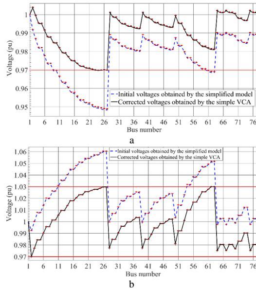
**Fig. 7.** The voltages obtained using simplified network component models as well as boxplots of initial and corrected voltages considering the uncertainty associated with shunt admittances of lines (a) in the voltage drop case, (b) in the voltage rise case
